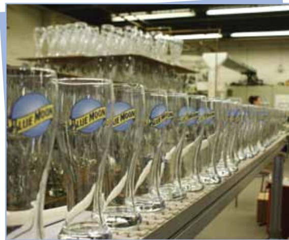
We are equipped to mass produce large orders with our fully automated machines. Glasses ride along the belt to be automatically loaded into the oven for firing.
