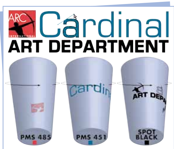
Artwork is separated into individual colors by our artists in preparation for being printed onto your glass
